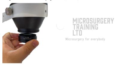
Attach 0.5X lens piece at base here to covert 10cm working distance to 15cm coupled with x2 X20 eyepiece lenses.
