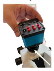
Screw on camera to adapter. Adjust camera focus and clarity by twisting the ring below the camera (arrow)
