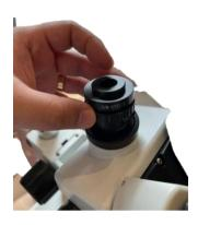
Screw on camera adapter at 3<sup>rd</sup> lens viewer socket
